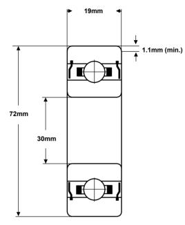
Material SAE52100 (rings & balls) chrome steel Material (cage) pressed steel Closures Metal shields Load rating (stat) 1541 Kgf 2717 Kgf Load rating (dyn) Speed Limit \* 10,000 rpm Standard Kyodo Yushi Lubrication \*\* Multemp SRL grease EMQ2 Extra Noise rating low noise
